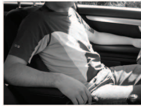
Fig. 2. Smart t-shirt used to register ECG and monitor heart rate. Electrodes are only felt during the initial minutes, after which the garment becomes
